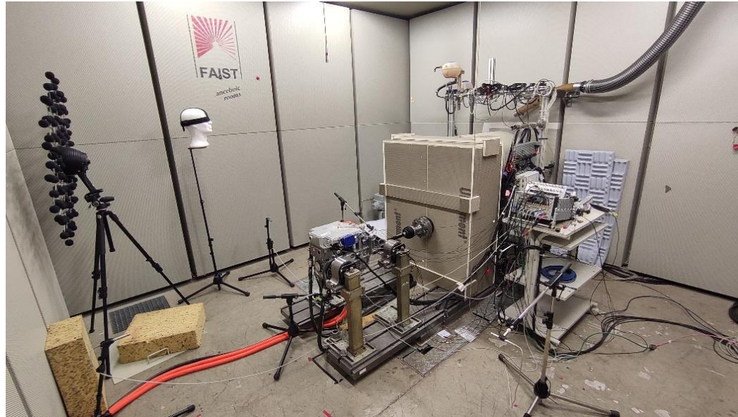
Test bench acoustic measuring system MKII (software PAK, Müller-BBM)
